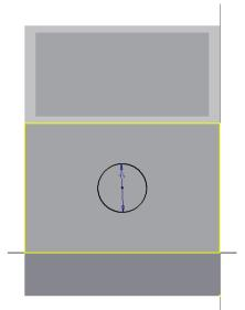
5. Finish the sketch and extrude the circle by subtraction 10mm.
