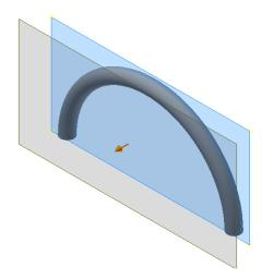
4. Sketch on the work plane and use the line tool to draw the profile shown.
