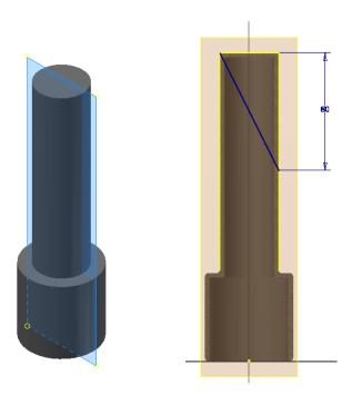
7. Extrude the profile by subtraction symmetrically through all material.
