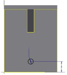
9. Finish the sketch and extrude the circle by subtraction all the way through the material.
