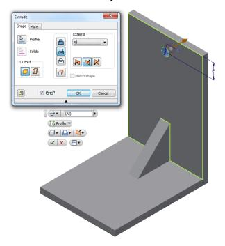
8. Select the bottom of the bracket and create a new sketch. Draw a circle 4mm and position it as shown.
