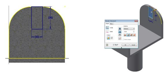
8. Create a work plane through the centre of the object and select the mirror tool. Select the extruded rectangle as the feature and the work plane as the mirror plane.
