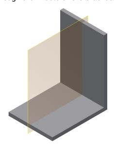
4. Create a new 2D sketch on this work plane. Use the line tool to draw a triangle and dimension it as shown.
