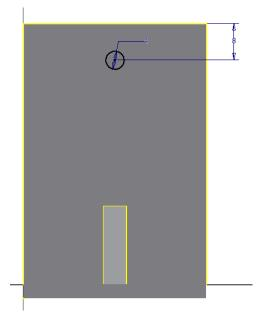
7. Finish the sketch and extrude the circle by subtraction all the way through the material.
